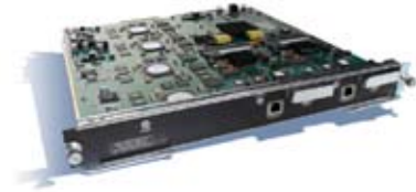
Catalyst 6500 Series/7600 Series Wireless Services Module (WiSM)
